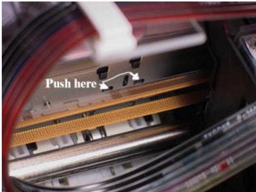
With a screw small driver – push in through these two holes (works one at a time) while pulling up on the sensor on the other side). Just above these holes see the catch feet of the sensor –
