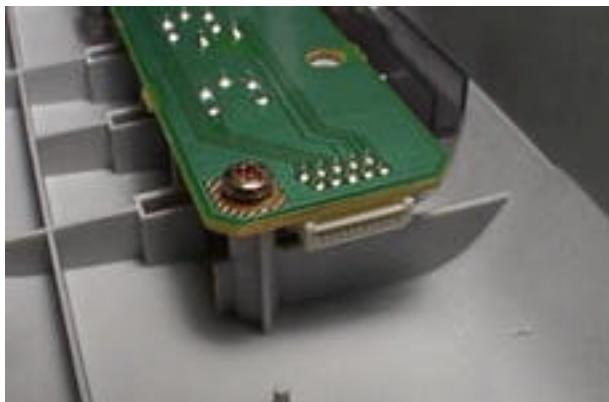
Bare Ribbon cable would be inserted in the plug (shown here with cable detached) that is the 4 switches in the top case. Ribbon slides in easy – blue side out. If you don't mind working with the loose cover in your way you could probably leave the ribbon cable attached.
