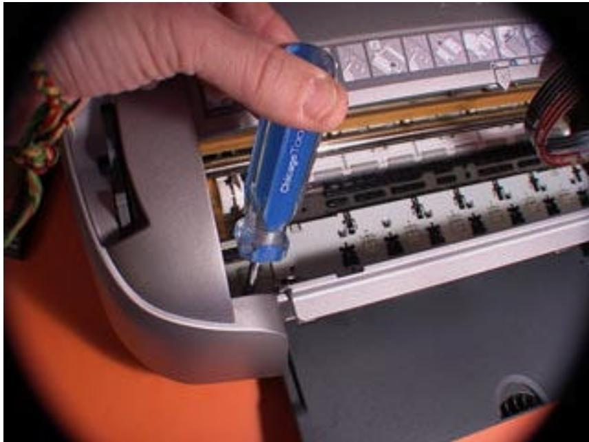
This is where the hidden catches are to release the case – both sides - use a flashlight!
